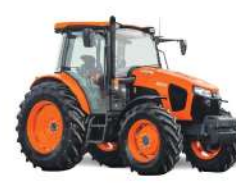
M5111, M5091 CAB/ARCO Motor: M5111: 115CV (CAB), 107CV (ARCO), M5091: 96CV (CAB), 94 CV (ARCO) Transmisión: 18A/18R (ARCO) ó 36A/36R con Dual Speed (CAB)
